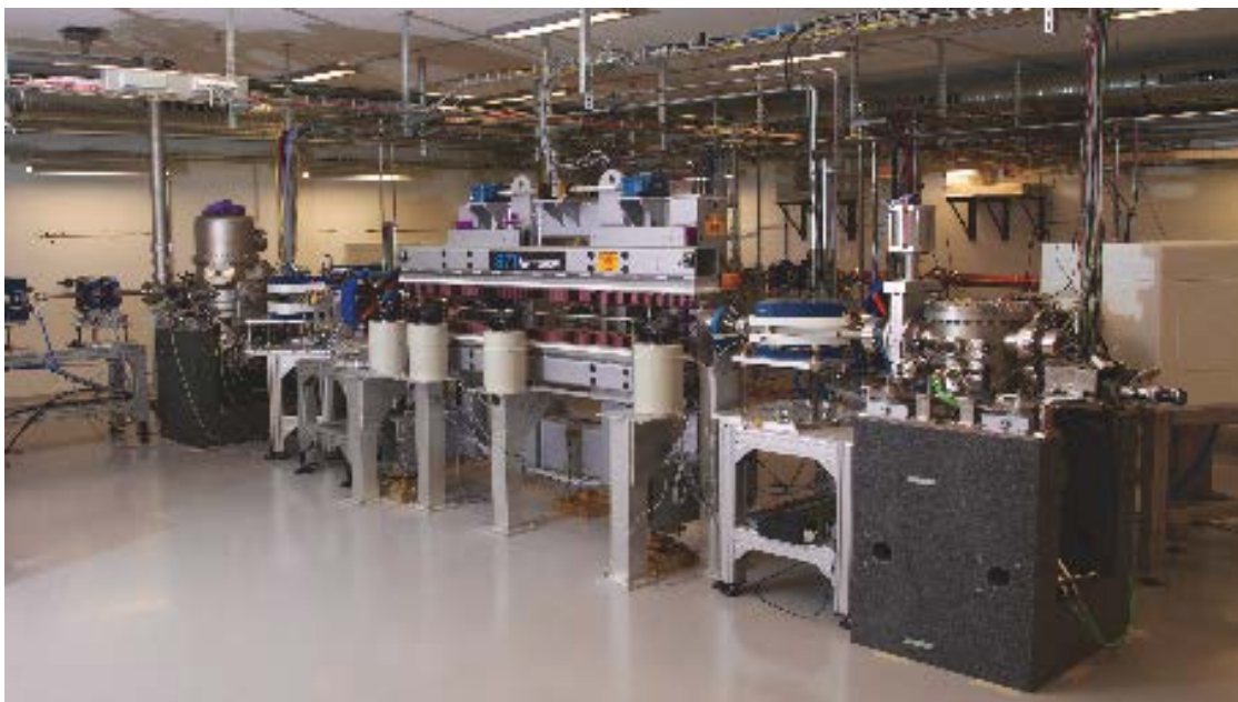
Figure 2: MIR FEL with undulator (center) and IR-cavity mirror chambers (left and right) as of 2013.
